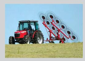
**ONE SINGLE-ACTING CYLINDER** folds both wings for easy transport (available on 1508, 1510 and 1512 models).
